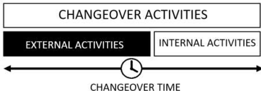
**Fig. 1.** - Internal and external operations – SMED.
