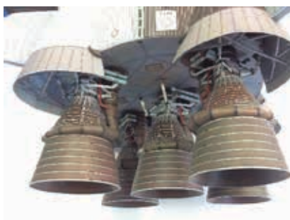
Detail trysek modelu rakety Saturn V
